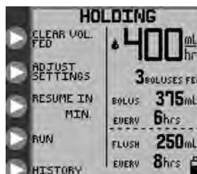
Figure 18B. HOLDING mode options, intermittent feeding mode.
